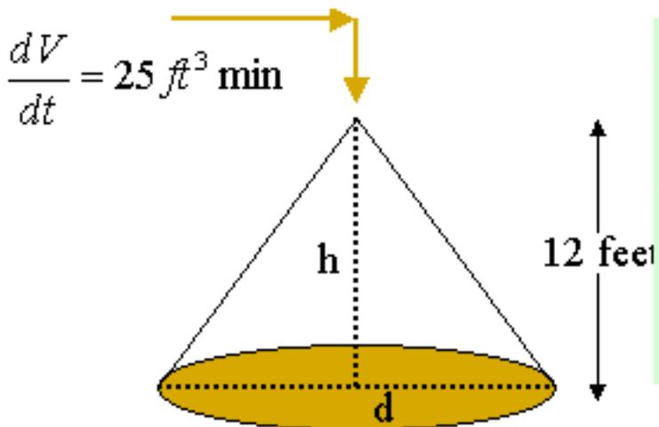
5. Water is leaking out of an inverted conical tank at a rate of 8,000 cubic meters per minute at the same time water is being pumped into the tank at a constant rate. The tank has a height of 12m and the diameter of the top is 4m. If the water is rising at the rate of 40 cm/min when the height of the water is 7m, find the rate at which water is being pumped into the tank. ( $8000 + 19.6\pi/9 \text{ m}^3 / \text{min}$ )
